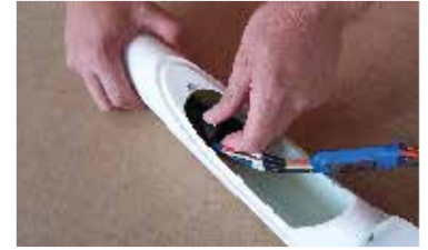
138. ...celek vsuneme do trupu... ... insert motor unit to the fuselage ...
