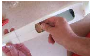
97. ... vsuneme podložku matic #2-31... ... insert rest for nut #2-31 ...
