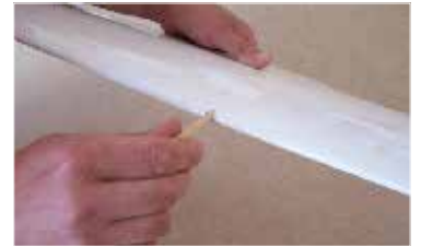
12. Kolík vsuneme do otvoru Push fixing pin to hole.
