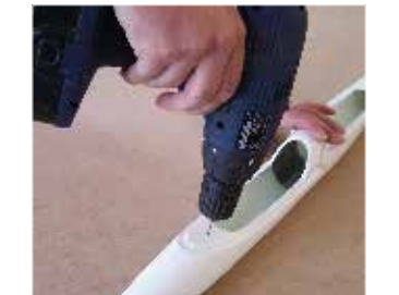
75. ...vyvrtáme otvor Ø2,2mm... ... drill hole ø 2.2 mm ...
