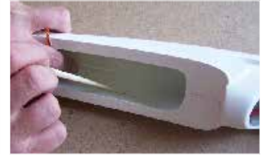
146. ...naneseme lepidlo... ... put glue on surface ...
