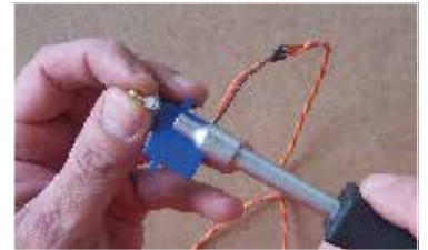
122. ...a zašroubujeme ... screw servo arm.
